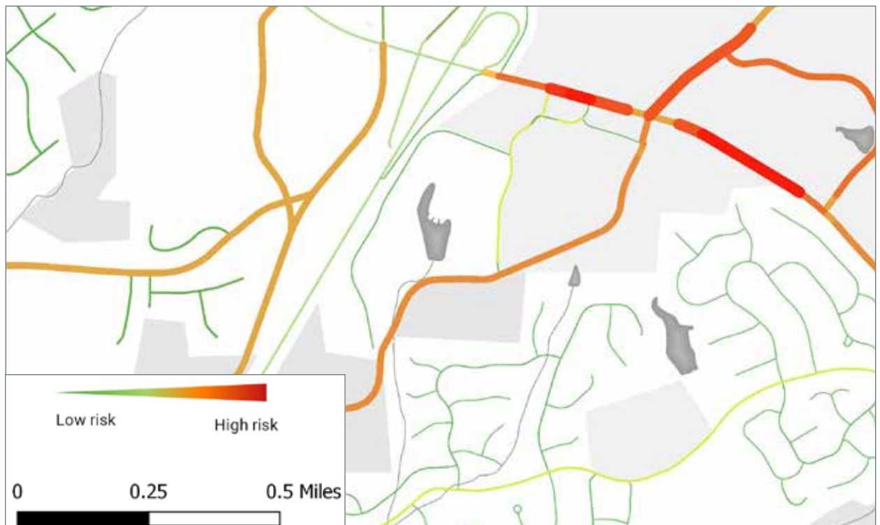
Pedestrian Risk Assessment map showing the relative risk of area roads based on roadway design elements, crash history, demand factors, and policy priorities.
