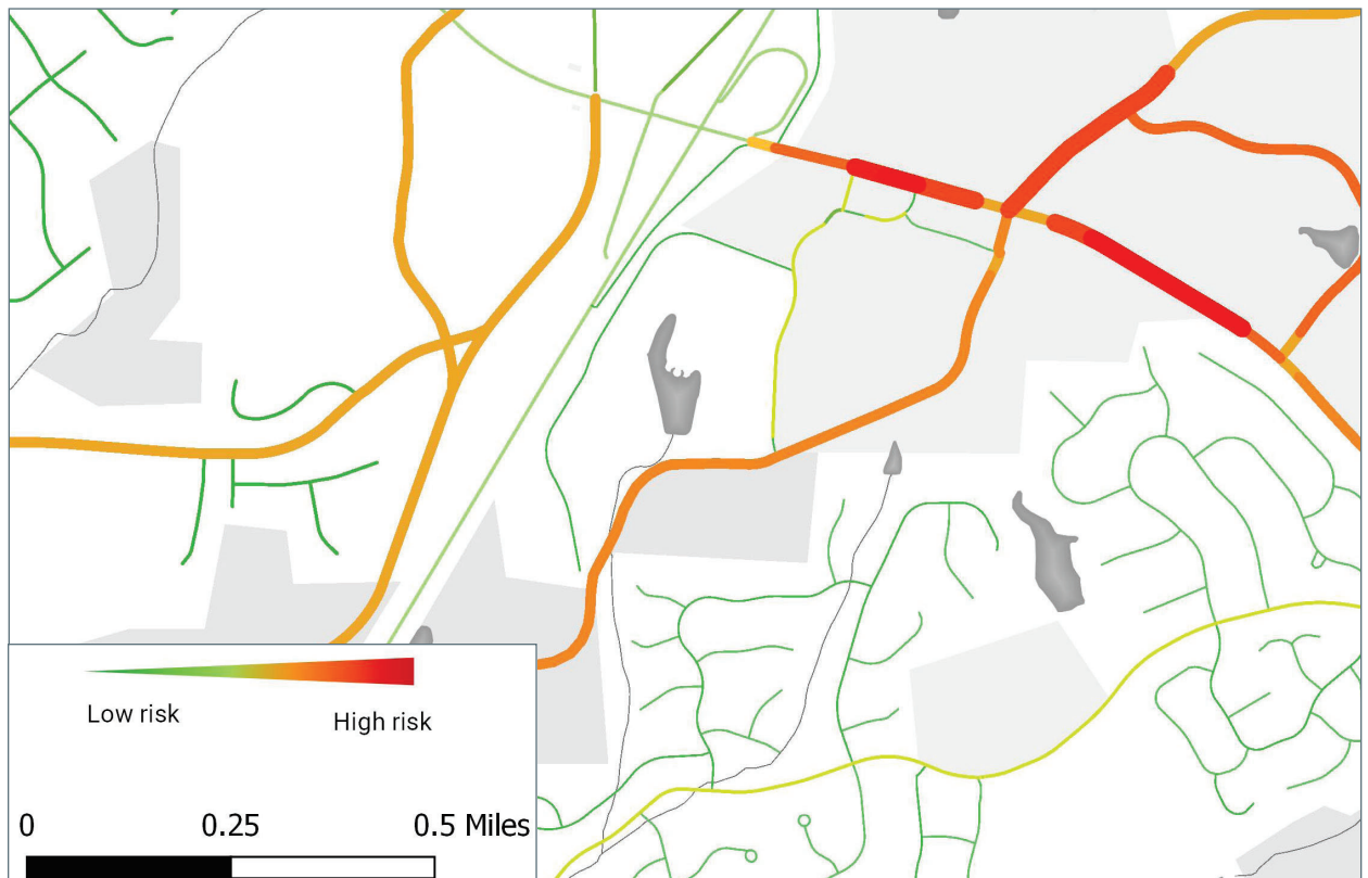
Pedestrian Risk Assessment map showing the relative risk of area roads based on roadway design elements, crash history, demand factors, and policy priorities.
