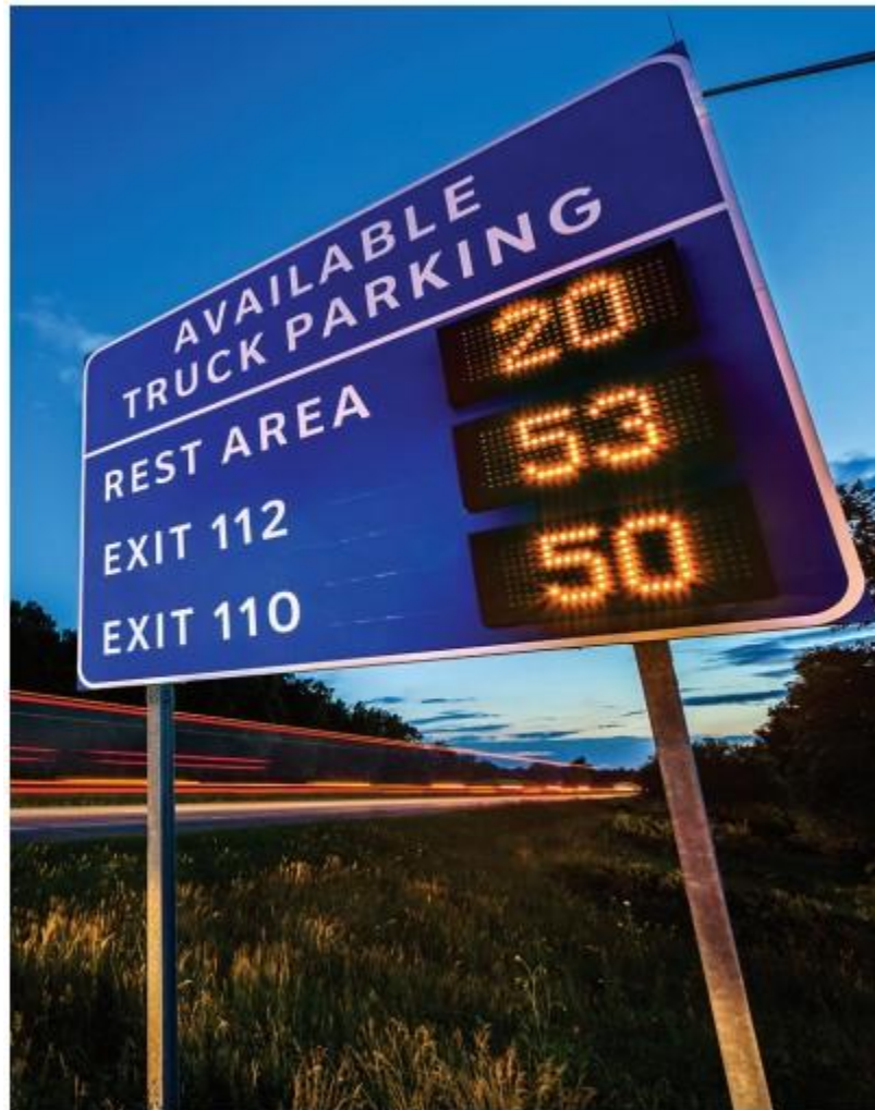
Figure 5: Dynamic Message Sign with Available Truck Parking
