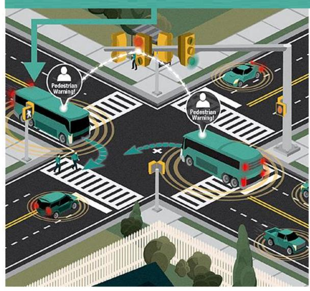
Warns drivers when a pedestrian is crossing the street as the vehicle is making a right or left turn.
